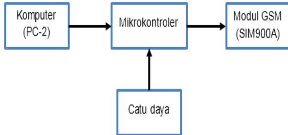
**Gambar 3. Blok diagram hardware**
