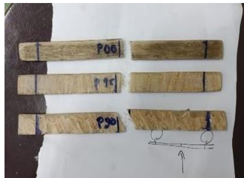
Figure 3. Fracture Results after Testing
