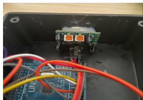
Gambar 8. Sensor PIR HC-SR501
