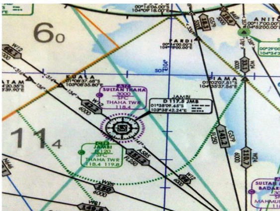
Gambar 2. ATS Route Sultan Thaha Jambi.
