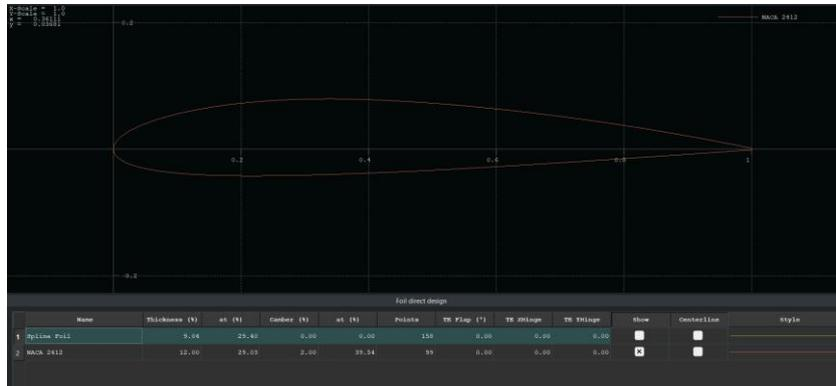
Gambar 3. Desain 2D Airfoil NACA 2412 , Xflr5
