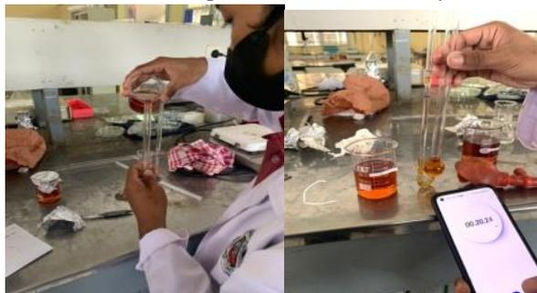
Gambar 8. Proses *pengujian Viscometer Ostwald*
